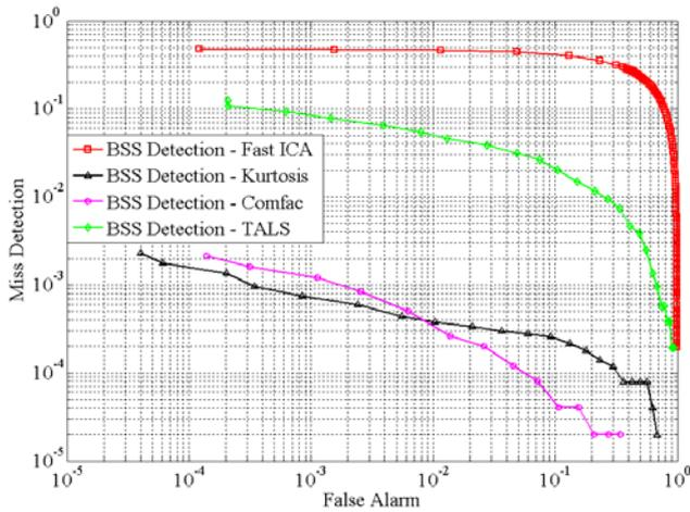
Figure 2. The miss-detection probability versus the false-alarm probability for the comparison between the proposed Kurtosis based spectrum sensing method and the other BSS methods. SNR=5dB, SUs number = 10 , CR transmitter is NOT in operation.
