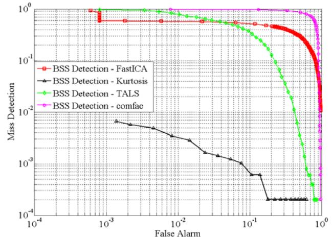
Figure 3. The miss-detection probability versus the false-alarm probability for the comparison between the proposed Kurtosis based spectrum sensing method and the other BSS methods. SNR=5dB, SUs number = 10 , CR transmitter is in operation.
